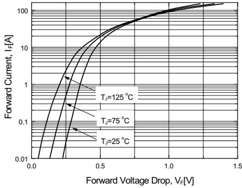
**Figure 1. Typical Forward Voltage Characteristics (per diode)**
